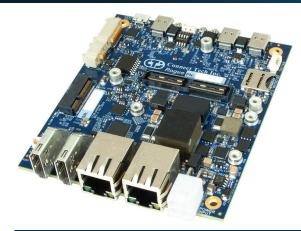
Rugged camera add-on expansion boards will also be available for use with the Rogue to interface directly with the Jetson AGX Xavier high density MIPI CSI interfaces.
