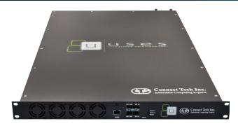
Includes Out of Band Management (OOBM) via an ARM-based SMARC module to control and monitor each of the Jetson TX2 modules.
