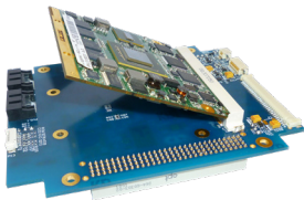
Note: Qseven CPU module mounted on bottom side. Qseven module sold separately.
