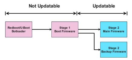
The Stage 1 firmware is independent of the Stage 2 (main) firmware and can be a different version.
