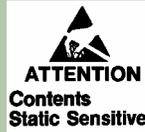
Your Titan/cPCI and Rear I/O adapters are very sensitive to static electricity. Make sure you wear an anti-static wristband before you remove the card from the anti-static shipping bag. When you remove the board from the anti-static bag, handle it only by the edges and place it on the anti-static bag or an anti-static mat.
