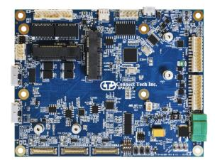
Spacely enables users to simultaneously connect up to 6 MIPI CSI-2 cameras as well as built-in expansion for GPS/GNSS.
