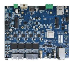
Cogswell also enables HDMI Video, USB 3.0, USB 2.0, USB OTG, Mini-PCle/mSATA expansion, and two RS-232 Serial Ports.
