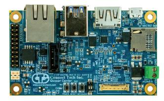
Quasar is ideal for robotic and unmanned applications that require the addition of MIPI, CAN, SATA or HDMI 2.0 ports.
