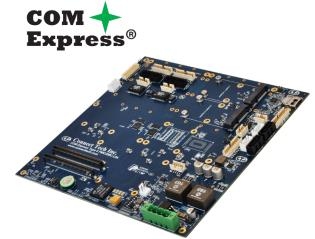
Ideal for military and aerospace applications, and accepts a wide input voltage range from a regulated or un-regulated source of +12V to +48V DC.
