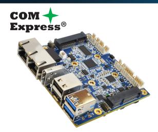
Ideal for space constrained applications and supports extended temperature ranges of -40°C to +85°C.
