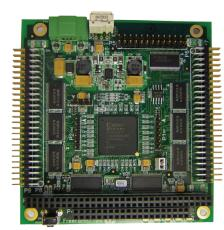
Connecting directly to the Digital I/O headers on the FreeForm/104, the "Daughter Board" also includes a PC/104 pass-through connector to allow the board to sit in-stack with the FreeForm/104 board.
