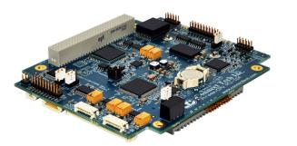
Xtreme/SBC conveniently provides on-board connectors allowing for instant access to a variety of features including SATA, Ethernet, USB, LVDS and VGA Video, RS-232 and RS-422/485.
