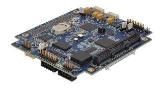
Xtreme/SBC conveniently provides on-board connectors allowing for instant access to a variety of features including SATA, Ethernet, USB, LVDS and VGA Video, RS-232 and RS-422/485.
