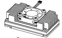
REMOVE PROTECTIVE FILM FROM THERMAL PAD APPLY ONE DROP OF LIGHT DUTY THREADLOCKER ON THREADS TORQUE FASTENERS TO 5.2 in-lb
