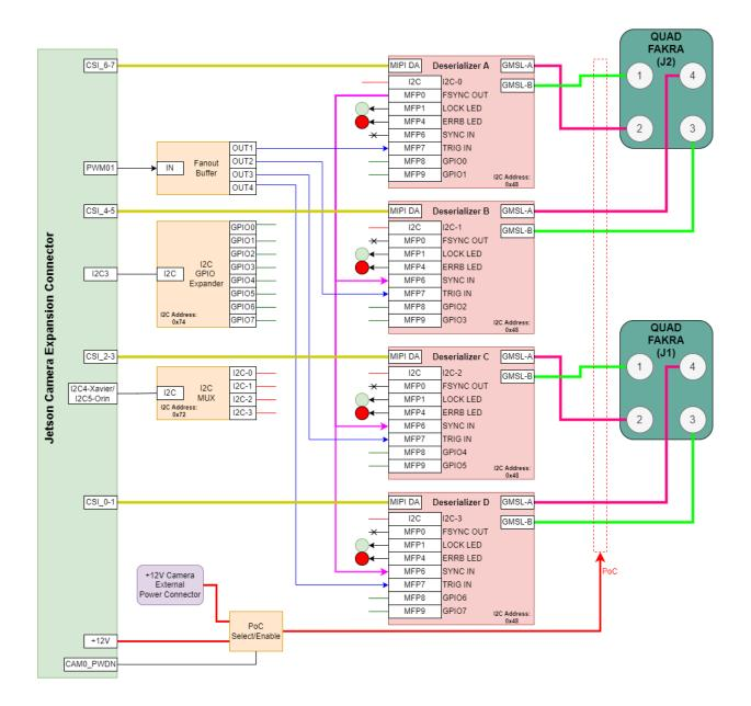
Note: The Power over Coax source is shared, but each GMSL port has its own filter which can handle up to 1.1A.
