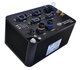
Rosie is designed to meet MIL-STD-810G as well as DO160G for shock and vibration along with ingress protection of IP68.
