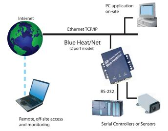
The Blue Heat/Net 2 enables you to connect any of your RS-232 or RS-422/485 serial devices directly to your Ethernet LAN.
