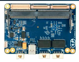
Quark's design includes a rich I/O set as well as positive locking IO connectors optimized for rugged environments.
