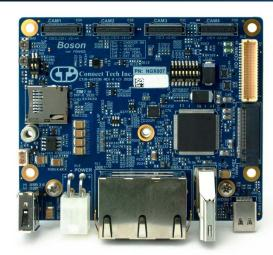
Equipped with 4x FRAMOS PixelMate connectors for instant access to the entire FRAMOS Sensor Module Ecosystem. Boson for FRAMOS has 2x Gigabit Ethernet, 2x USB, and 4x MIPI connections, and is almost 30% smaller than the Xavier NX Developer Kit.
