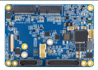
Hadron's design includes a wide input voltage, rich I/O set as well as locking IO connectors optimized for rugged environments.
